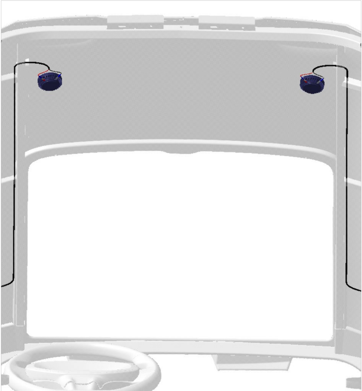
View from the bottom of the car pavillon with the two exciters installed.
